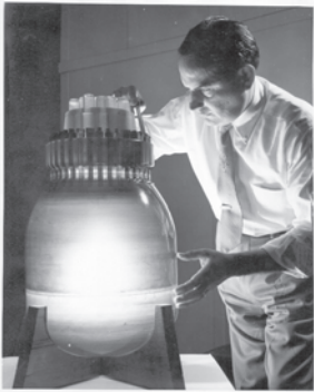
Milt Leven with a large epoxy model of a reactor pressure vessel
