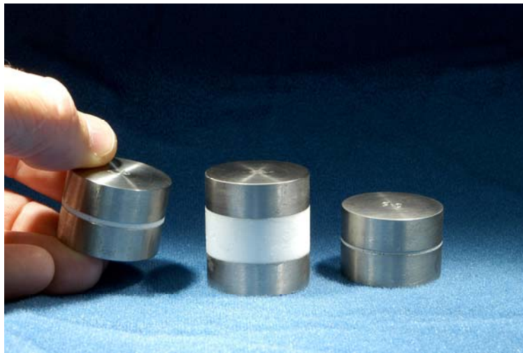
Figure 2 - Calibration Test Hardware for Young's Modulus and Poisson's Ratio
