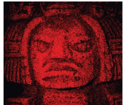
Portion of Mayan figure photographed under helium-neon laser illumination at f -22 aperture. The intrusive effects of subjective laser speckle are apparent. Digital photograph by Gabriel Isaicu of Michigan State University, Mechanical Engineering Department, January 2007.
